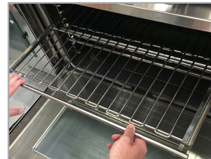
7 Once properly installed you will be able to slide rack out, and the guard rail hook will prevent the rack from coming out of the oven completely for safety purposes.
