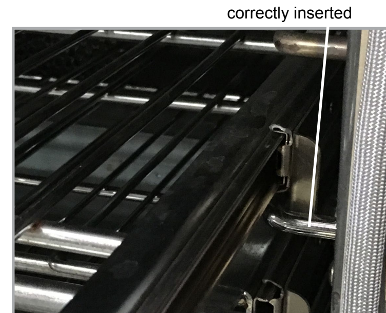
6 Close up image of the slide rail of rack correctly inserted into the front ladder system.
