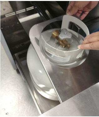
Once the LP Tank Harness of fitted over the LP cylinder collar as shown, screw the included LP regulator hose assembly to the LP tank, open LP cylinder top valve and check for system leaks before lighting the grill
