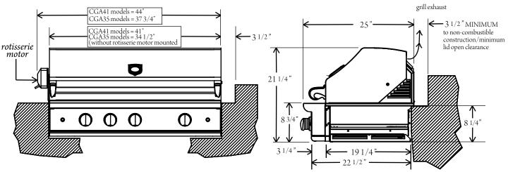
Important! Gas fittings, regulator, and installer supplied shut-off valves must be easily accessible.
