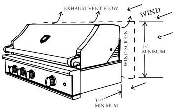
NOTE: If wind against the rear of the unit is an issue, a wind screen should be added behind the grill to block rear wind. The non-combustible wind screen should be built taller than the top of the flue opening at the back of the grill (15" min) and have a clearance of a minimum of  $3\ 1/2$ " from the rear of the grill as shown above.
