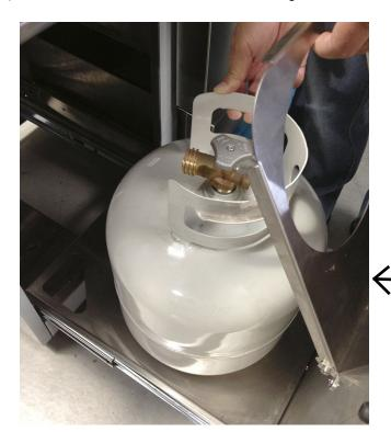
Fold down LP Tank restraint harness over top of the LP tank as shown
