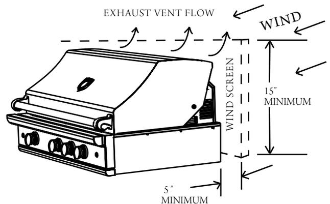
NOTE: If wind against the rear of the unit is an issue, a wind screen should be added behind the grill to block rear wind. The non-combustible wind screen should be built taller than the top of the flue opening at the back of the grill (15" min) and have a lid opening clearance of a minimum of 5" from the rear of the grill as shown above.
