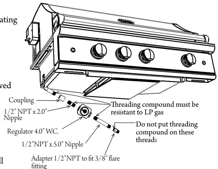
\*Installation must conform with local codes or with the National Fuel Gas Code ANSI Z223.1 or the CAN/CGA Propane Installation Code
