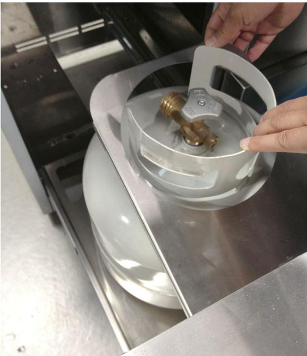
← Once the LP Tank Harness is fitted over the LP cylinder collar as shown, screw the included LP regulator hose assembly to the LP tank, open LP cylinder top valve and check for system leaks before lighting the grill
