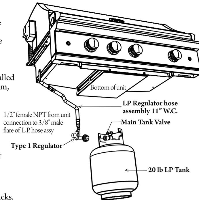
\*Installation must conform with local codes or with the National Fuel Gas Code ANSi Z223.1 or the CAN/CGA-B149.2 Propane Installation Code
