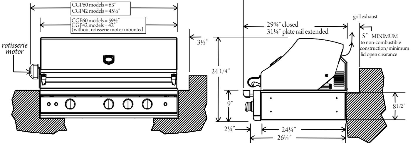
Important! Gas fittings, regulator, and installer supplied shut-off valves must be easily accessible.
