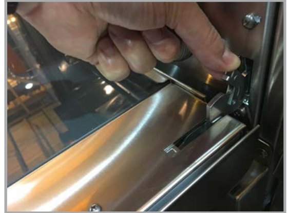
Fig. 4a Hinge retainer clip comes down for the unlocked position
