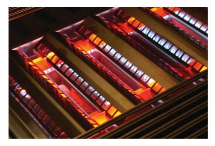
Crossflame patented radiant system utilized on both Crossflame burner designs.
